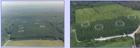
Figure 1. Free-air CO 2 enrichment experiments (FACE) where plots in an intact loblolly pine forest (left) and an intact sweetgum forest (right) are exposed to ambient (~370 μl l -1 ) and elevated (~570 μl l -1 ) atmospheric CO 2 .
