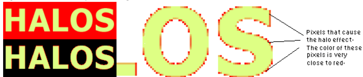
Figure 5. "Halo" caused by anti-aliasing.
