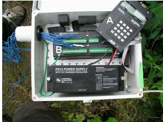
Figure 2.1 The CR-10X data logging unit used in mapping out the temperature profile of the compost pile. The control keypad (A) was used to set the sampling rate and program. Temperatures were recorded as voltage measurements in the actual DLU (B).
