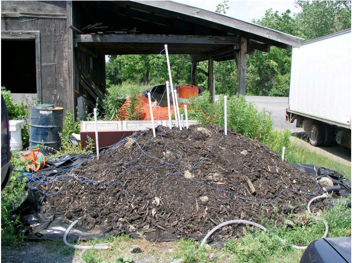
Figure 2.3 A photograph of the compost pile after the PVC sheathes and thermistors had been inserted. Originally five depth probes and five lateral probes were used to get precise temperature readings from a variety of locations within the pile. In this photograph one of the lateral probes was removed to measure atmospheric temperature.
