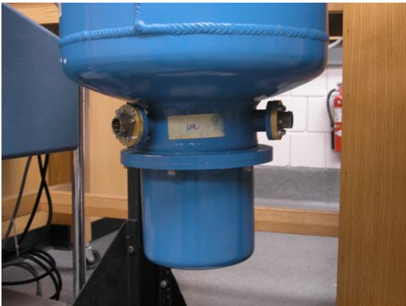
Figure D.2 Picture of the bottom of the Dewar / Vacuum Chamber used in CNS 211 for all measurements.
