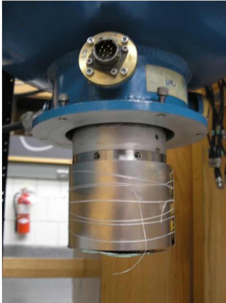
Figure 2.5 Picture of the outer IR shield attached to the bottom of the dewar
