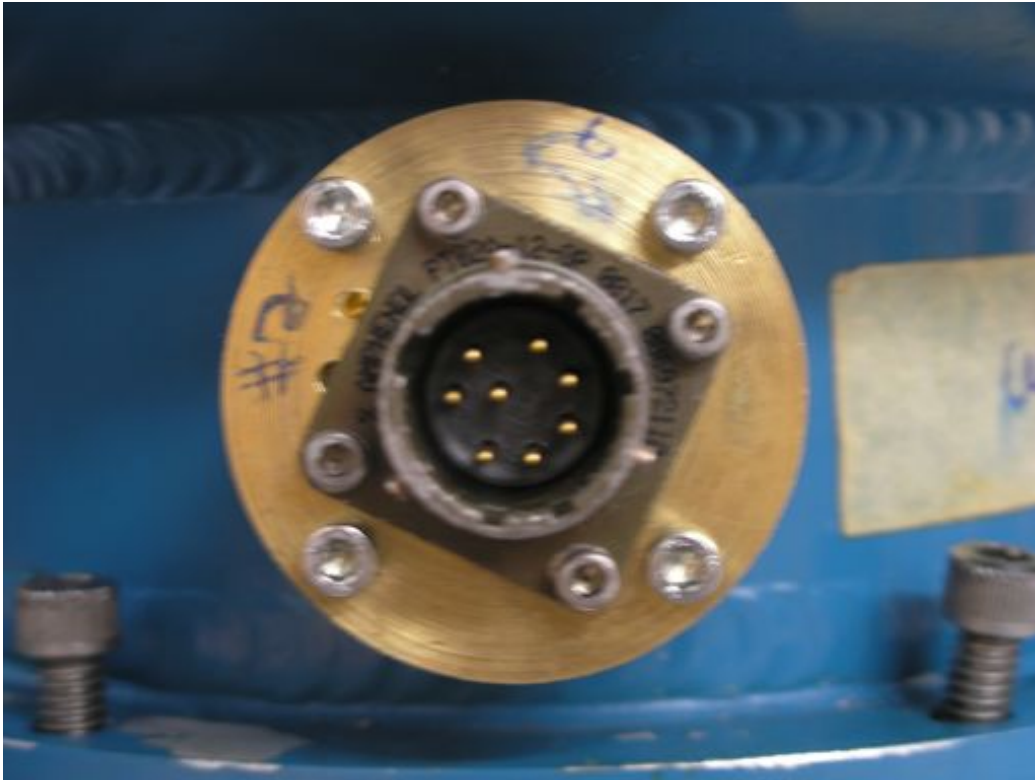
Figure 2.4 Picture of one of the Vacuum feedthroughs fabricated to fit onto the Dewar in CNS 211
