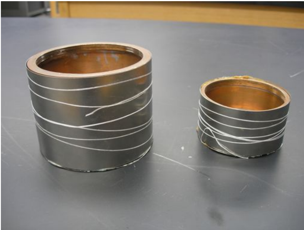
Figure 2.6 Picture of both IR shields outside of the dewar
