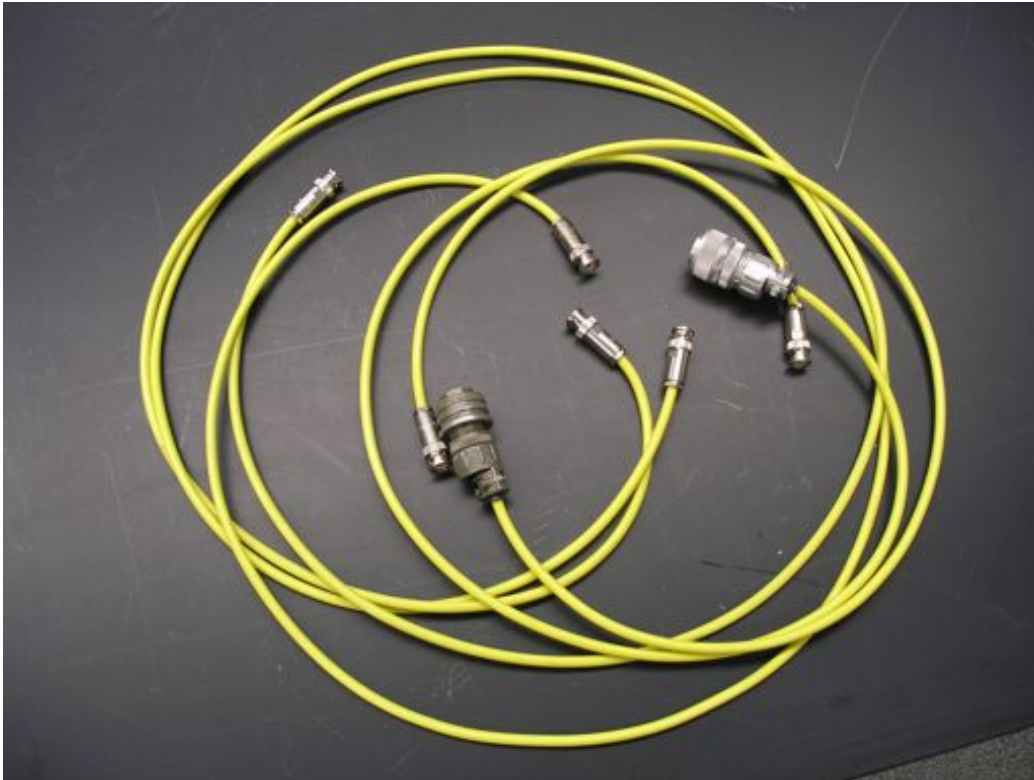
Figure 2.8 Picture of some of the Tri-Ax wires that were made for this project
