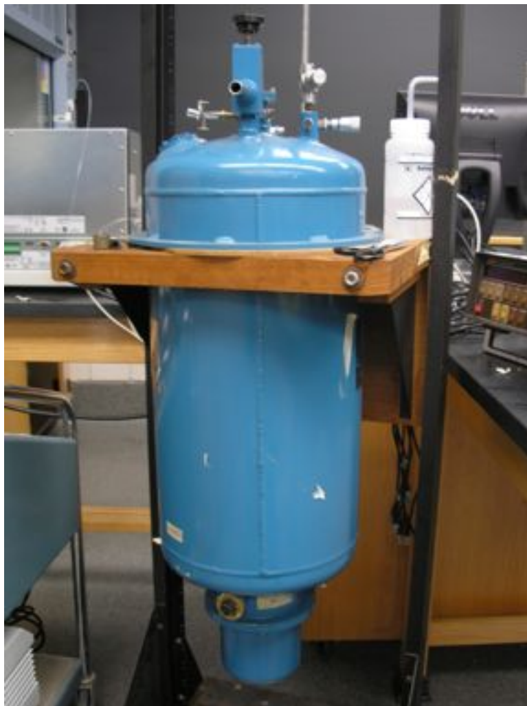
Figure 2.3 Picture of the Dewar / Vacuum Chamber used at IC for some measurements
