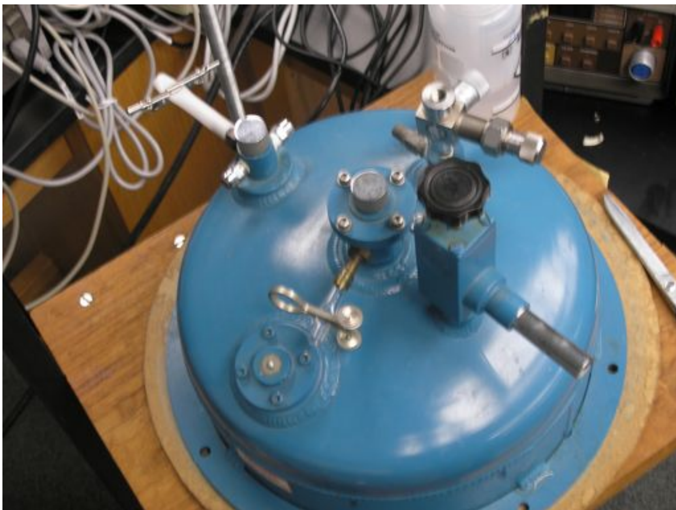
Figure D.1 Picture of the top of the Dewar / Vacuum Chamber used in CNS 211 for all measurements.
