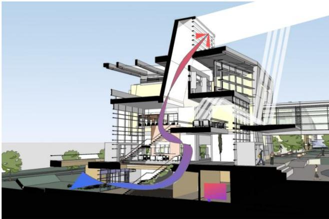
The central atrium and light monitor act as a solar chimney. The energy management system controls operable windows, inducing stack effect when exterior conditions are appropriate. CO<sub>2</sub> monitors additionally help control indoor air quality and also save energy, turning the ventilation fans on only when the building needs to vent stale air.
